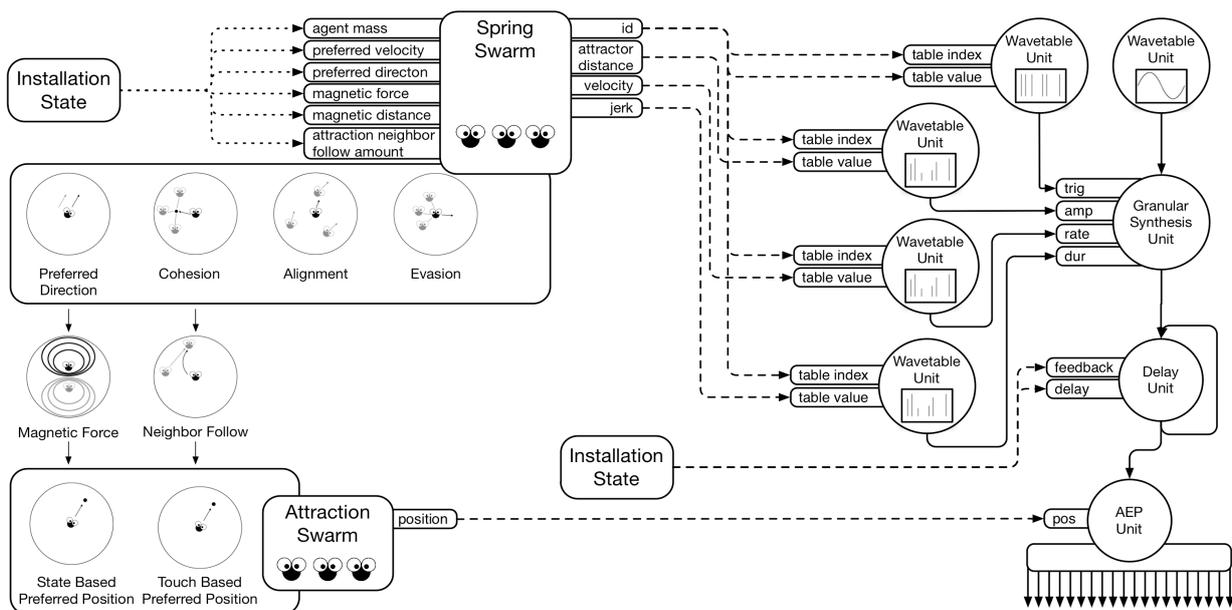
**Figure 4.** Schematics of the swarm music example entitled "Flow". The characteristics of the swarm simulation are depicted on the left side. The musical architecture is shown on the right. The dsp chain is shown a solid arrows. The mapping relationships between the swarm simulation and the music engine is depicted as dashed arrows.
