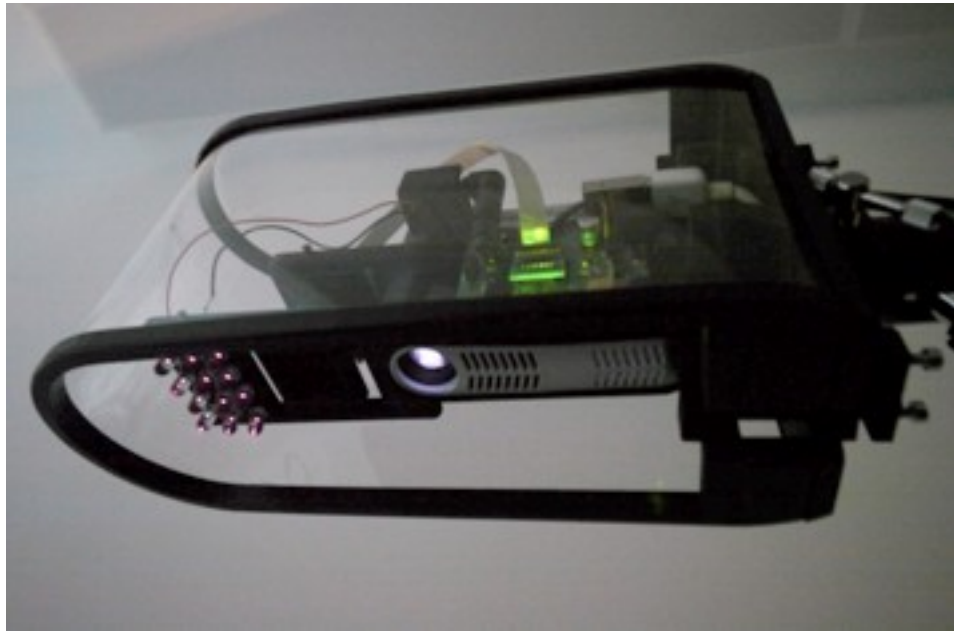
Figure 2: Cycles Installation Detail. The photo shows the structure that houses a video projector, a camera and an infrared light source.
