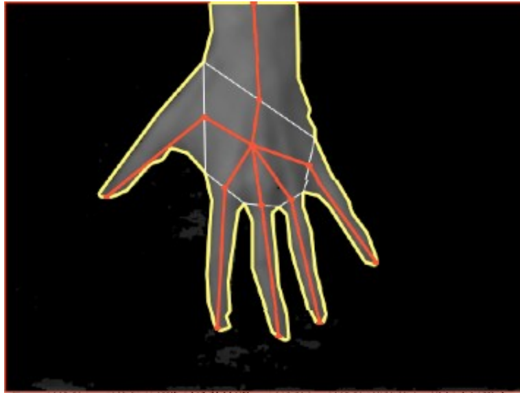
Figure 3: Hand-Tracking Software. The screenshot depicts the hand's contour as yellow lines, the fingers' and wrist's orientation as red lines, and the boundaries of the palm as gray lines.
